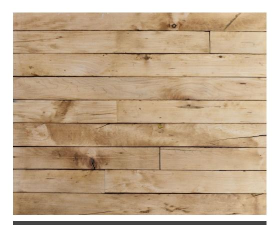
Species: Maple Thickness: 3/4" Widths: 2 1/4 and 3" widths Lengths: Random lengths from 3' - 10' Profile: T&G Surface: Planed Character: Nail holes, pin knots, occasional scars Applications: Floors, walls, and ceilings
